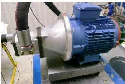
Fig. 2. Motor-pump unit coupled to its loading mass.
