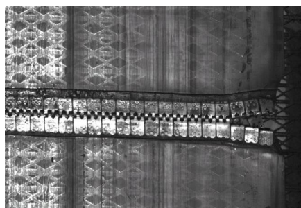
Fig. 2. Mechanical failure of steel belt joint[7].
