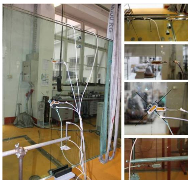
Fig. 5. Strain measuring points
