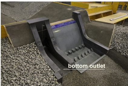
Fig. 1: Dam and bottom outlet, full model, downstream view
