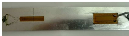
Fig. 1. Resistive strain gauge (on left) and piezo sensor (on right) bonded to aluminum alloy sample.
