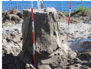
Fig.3 Excavated cemented sand column.
