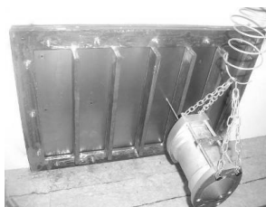
Fig. 2. Experimental model of periodically supported panel with an axial exciter Schenck VibroPower 41
