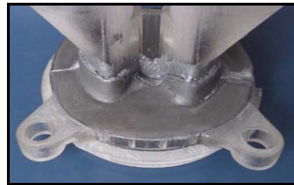
Fig. 4: Optical photostress coating layered RPT valve housing
