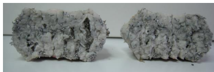
Fig. 5. Cross-section of compressed specimen showing conical deformation distribution
