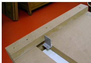
Fig. 6. The detail of deep girder reliance of model 1.
