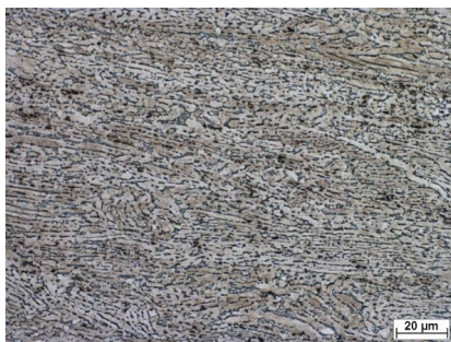
Fig. 1. Microstructure of Grade 5 Ti alloy, HNO 3 +HF+glycerine [6]
