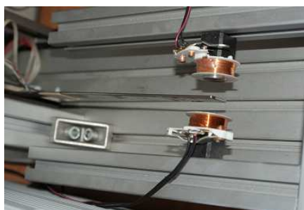
Fig. 2. A pair of electromagnetic inductors used for excitation of the analysed system.
